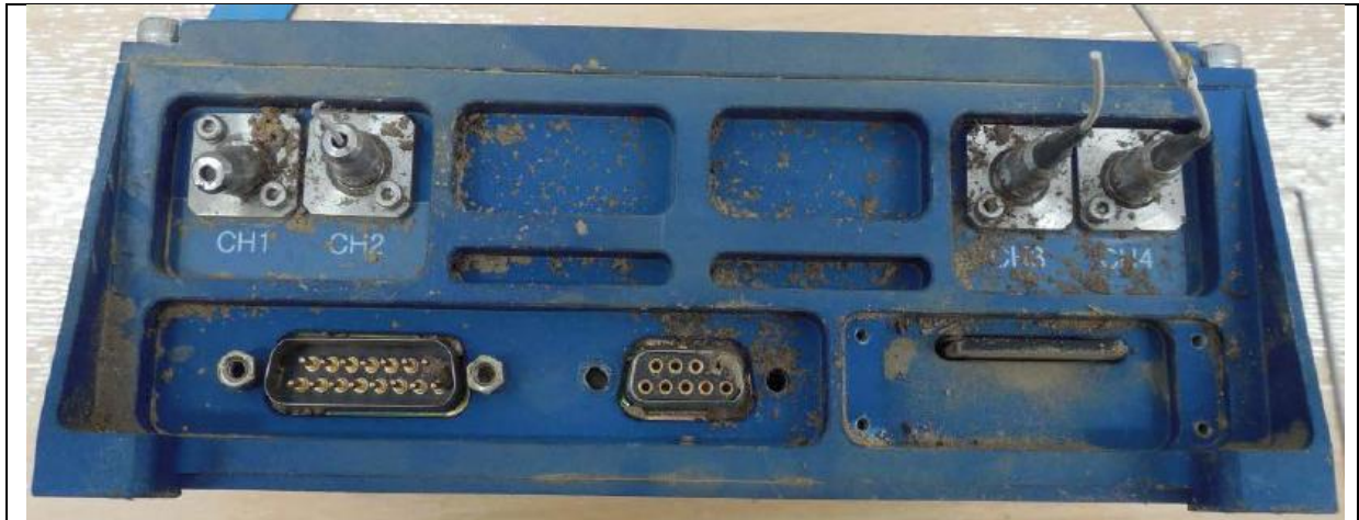
Fig. 13: Details of the Interrogator front with the connectors, three of them having their fibers still attached
